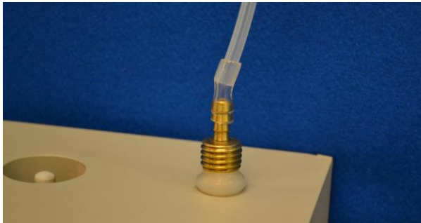
Figure 5. VAPOR PIN® sampling device sample connection
