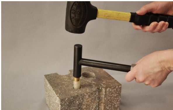
Figure 2. Installing the VAPOR PIN®
