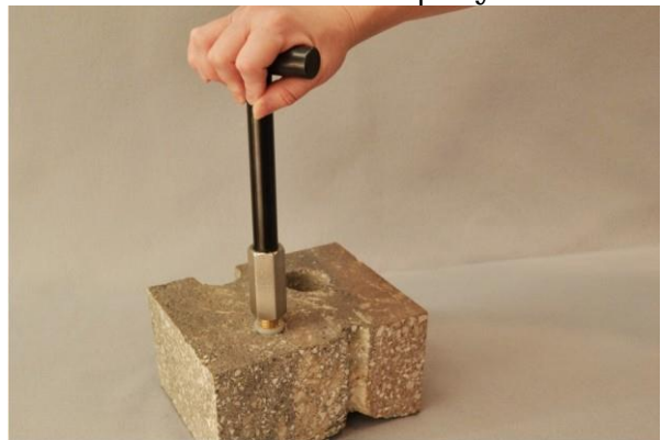
Figure 7. Removing the VAPOR PIN® sampling device
