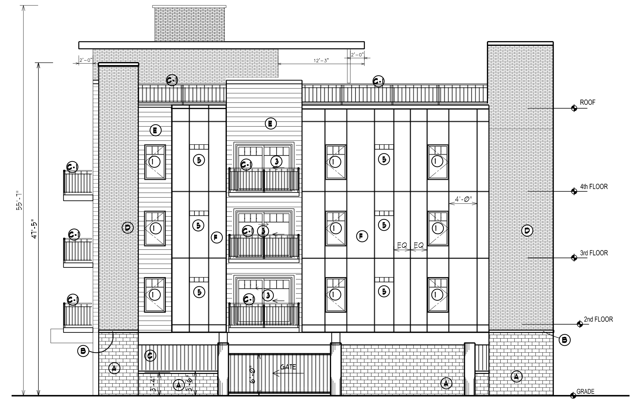
RIGHT SIDE (NORTH) ELEVATION 1/8" = 1'-0"
