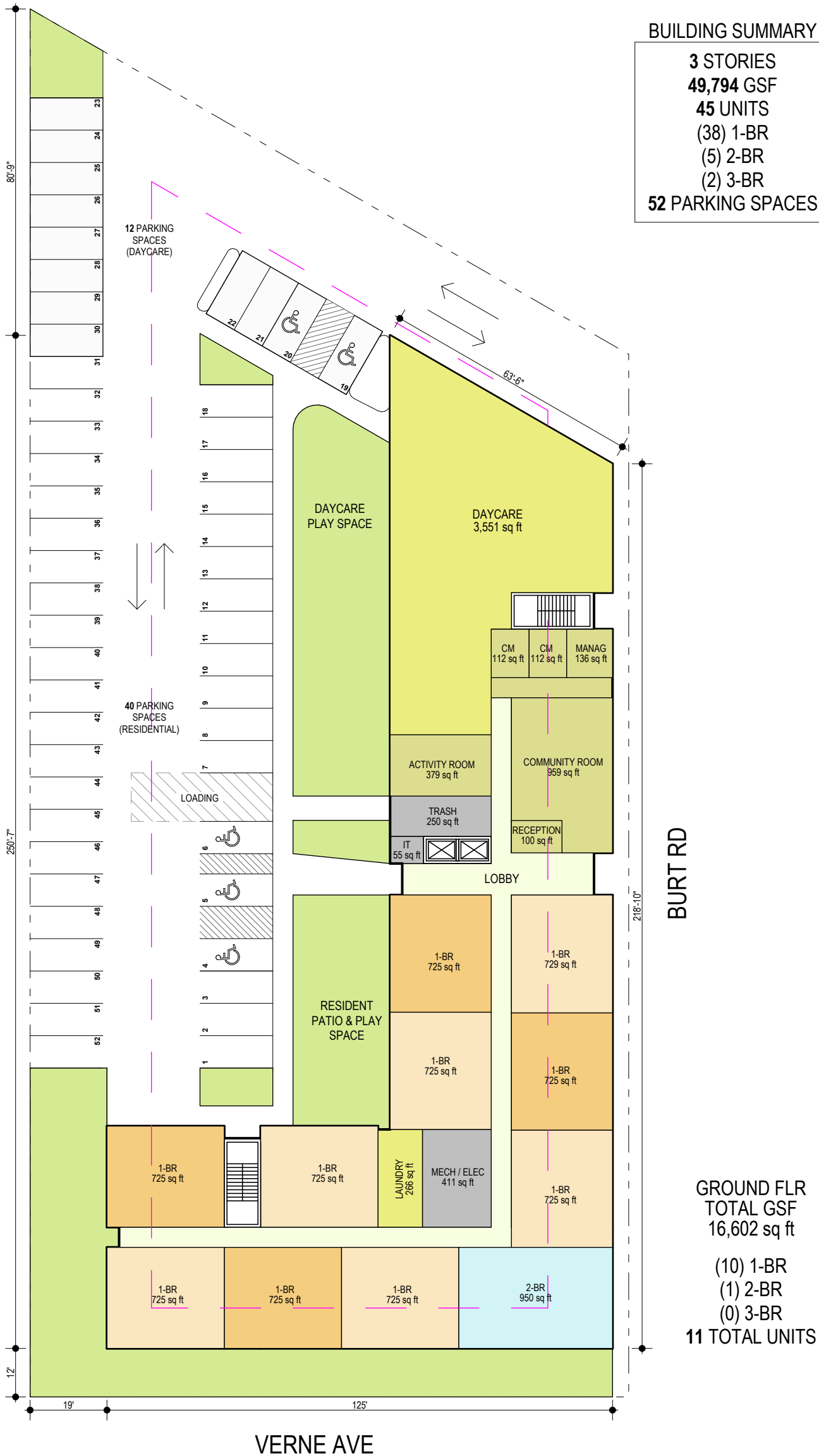
Site & Ground Floor Plan SCALE: 1" = 30'
