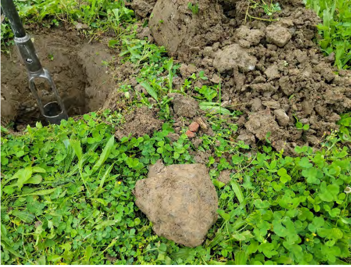
View of Typical Debris Found in Boring
