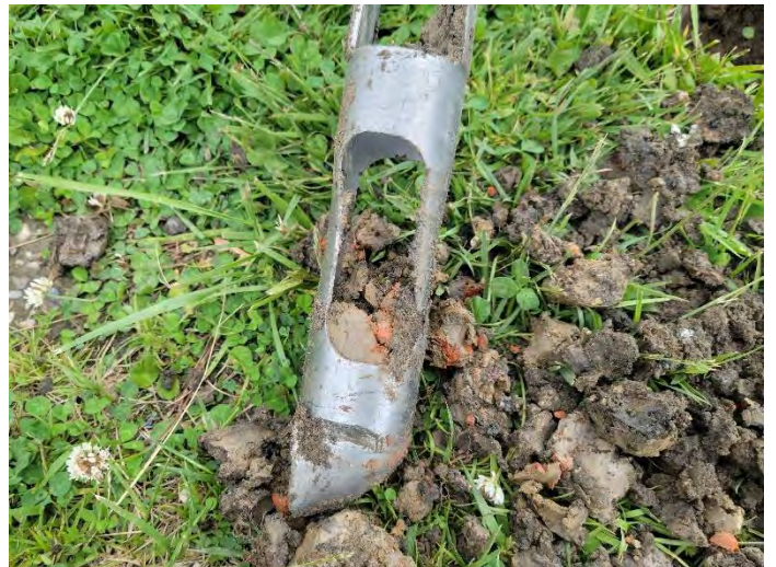
View of Debris in Auger
