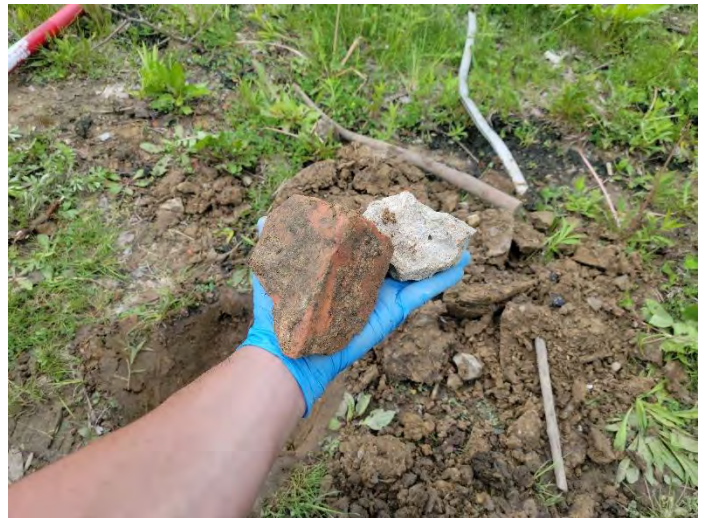
View of Typical Debris Found in Boring
