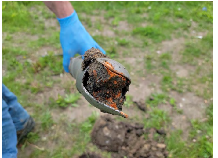
View of Brick Debris on Soil Auger
