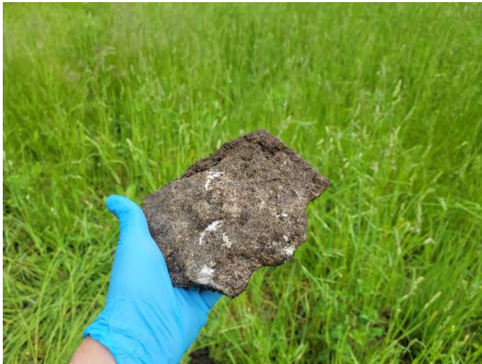
View of Typical Debris Found in Boring
