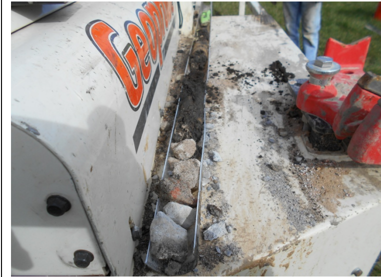
Photo 4. Urban debris in a core from soil boring SB-3
