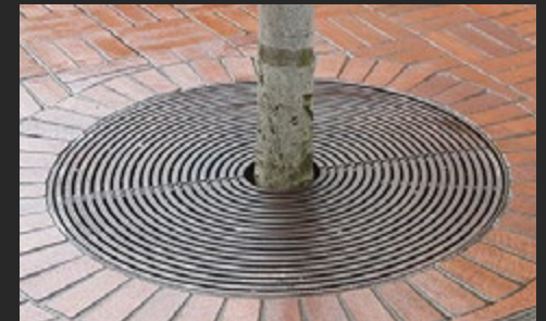
Urban Accessories 'Rainbow' 7 ft. dia. round 16" diameter opening Cast Ductile Iron with Baked on Oil-finish Load Class C ADA compliant
