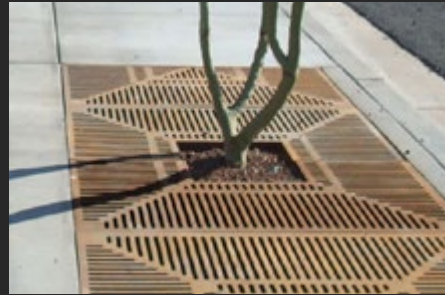
Ironsmith 'ADA' 4ft. x 12ft. 12" x12" opening Cast Ductile Iron with Baked on Oil-finish Load Class C ADA compliant
