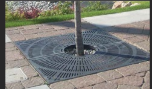
EJCO 'Sunray' 4ft. x 12 ft. 12" radius opening Cast Ductile Iron with Baked on Oil-finish Load Class C ADA compliant
