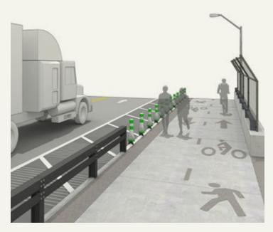
Dimensional constraints limit path width in this section. The proposed configuration allows adequate space for large trucks to maneuver while keeping greenway users safe. Rumble strips adjacent to the cycle track warn drivers of their proximity to the edge of the roadway, further enhancing user safety.
