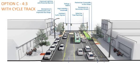
4:3 Lane Conversion Road-Grade Cycletrack Buffer Between Cycletrack and Parking with Traffic Bollards
