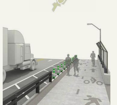
Dimensional constraints limit path width in this section. The proposed configuration allows adequate space for large trucks to maneuver while keeping greenway users safe. Rumble strips adjacent to the cycle track warn drivers of their proximity to the edge of the roadway, further enhancing user safety.
