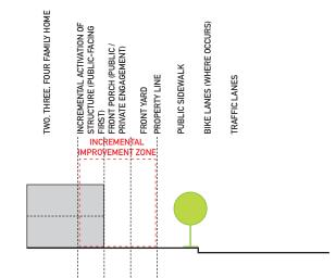
**Activated Edges Section Diagram**
