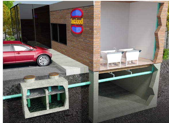
Periodic inspection and cleaning of grease trap(s) in commercial kitchens should be part of an overall maintenance program to reduce risk to employees and customers and prevent clogging sewer pipes.
