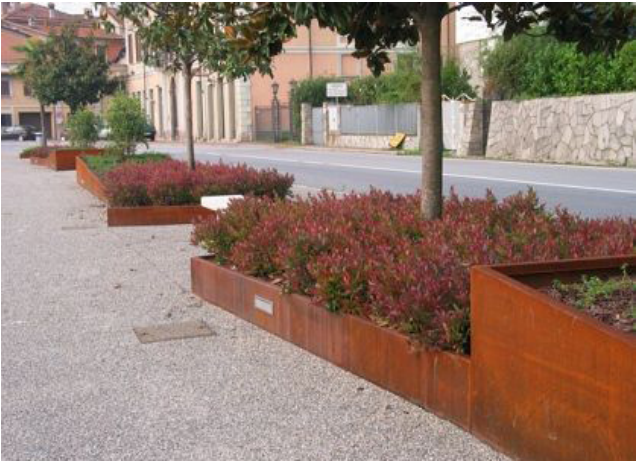
③ Private Streets Elevated planters and at grade plantings to manage street run-off and provide screening
