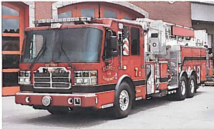
Platform Ladder Truck
