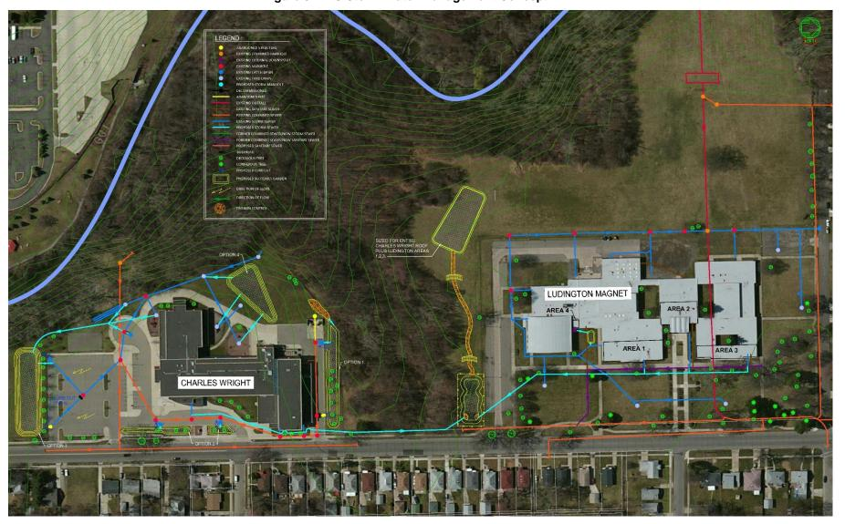
Figure 9 DPS Storm Water Management Concept 2
