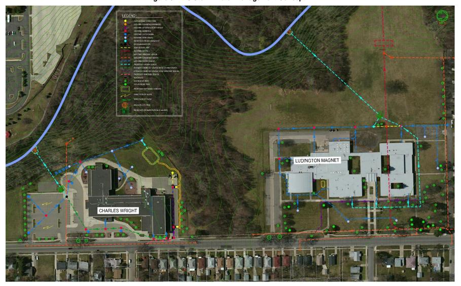
Figure 8 DPS Storm Water Management Concept 1
