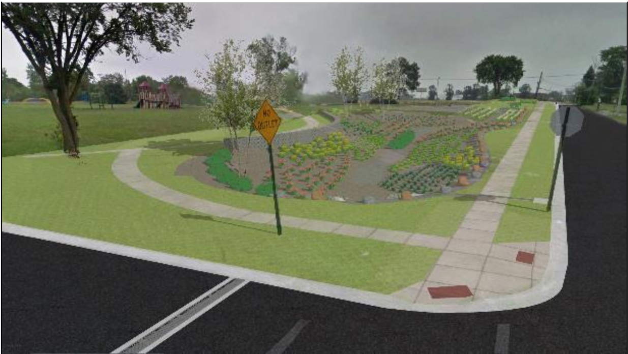
Figure 26 O'Shea Park Bioretention Improvement Rendering
