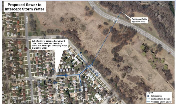
Location of existing and new storm sewer pipes on Constance Street
